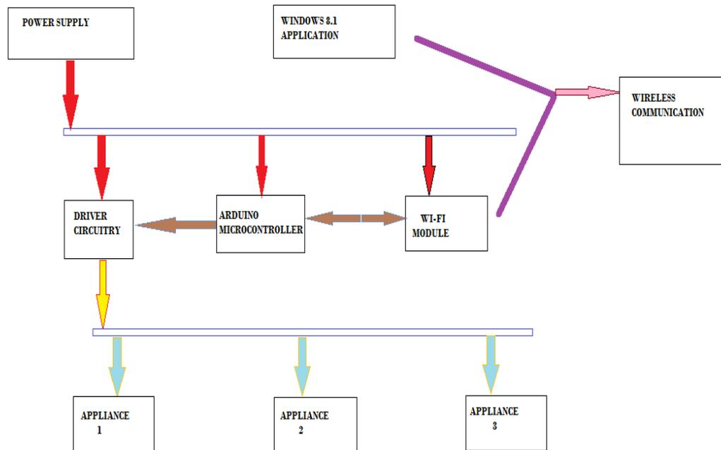
**Figure1: Activity diagram of HAS system**
